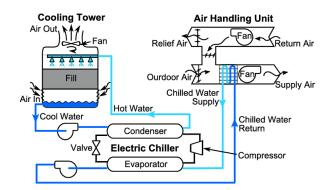
A chiller (cooling water circulation device) is a general term for a device that controls the temperature by circulating a liquid such as water or heat medium as a cooling liquid whose temperature was adjusted by the refrigerant cycle.
