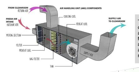
The air handling unit (AHU) is the heart of central air conditioning. It collects outside air and room air, removes dust and other particles from the collected air, adjusts the temperature and humidity and then supplies comfortable and refreshing air-conditioned air into the rooms through ducts.
