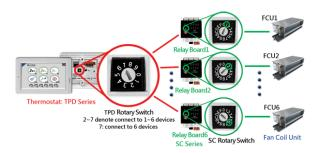
A fan coil unit (FCU) contains a fan which draws the air in a space into the unit then blows it over a cooling or heating coil. The air comes out of the FCU either cooler or hotter than before. They are used in some office buildings and shopping centres and typically specified where there are multiple small spaces requiring individual control.
